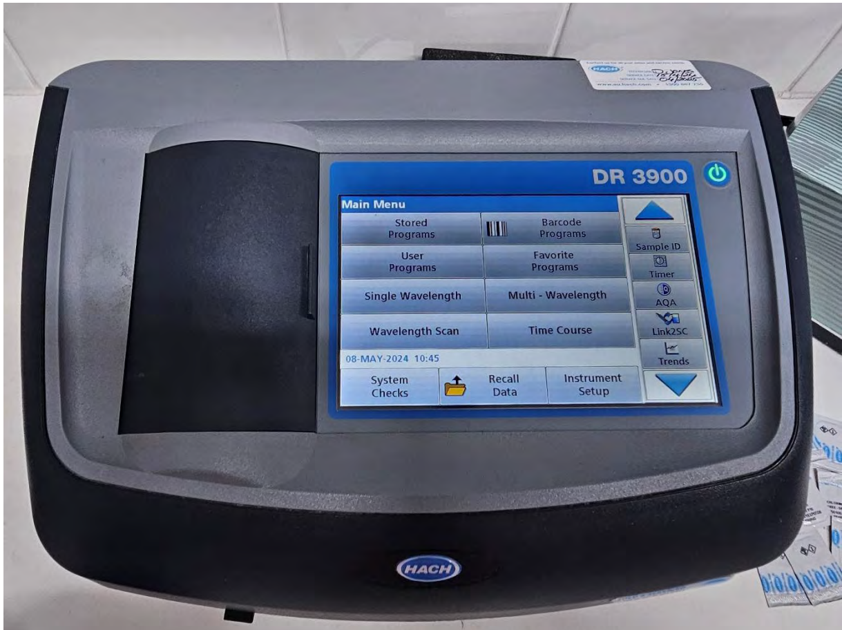
Photo 11: HACH DR3900 – Used by WTP Operator for fluoride testing as backup instrument at Moranbah WTP
