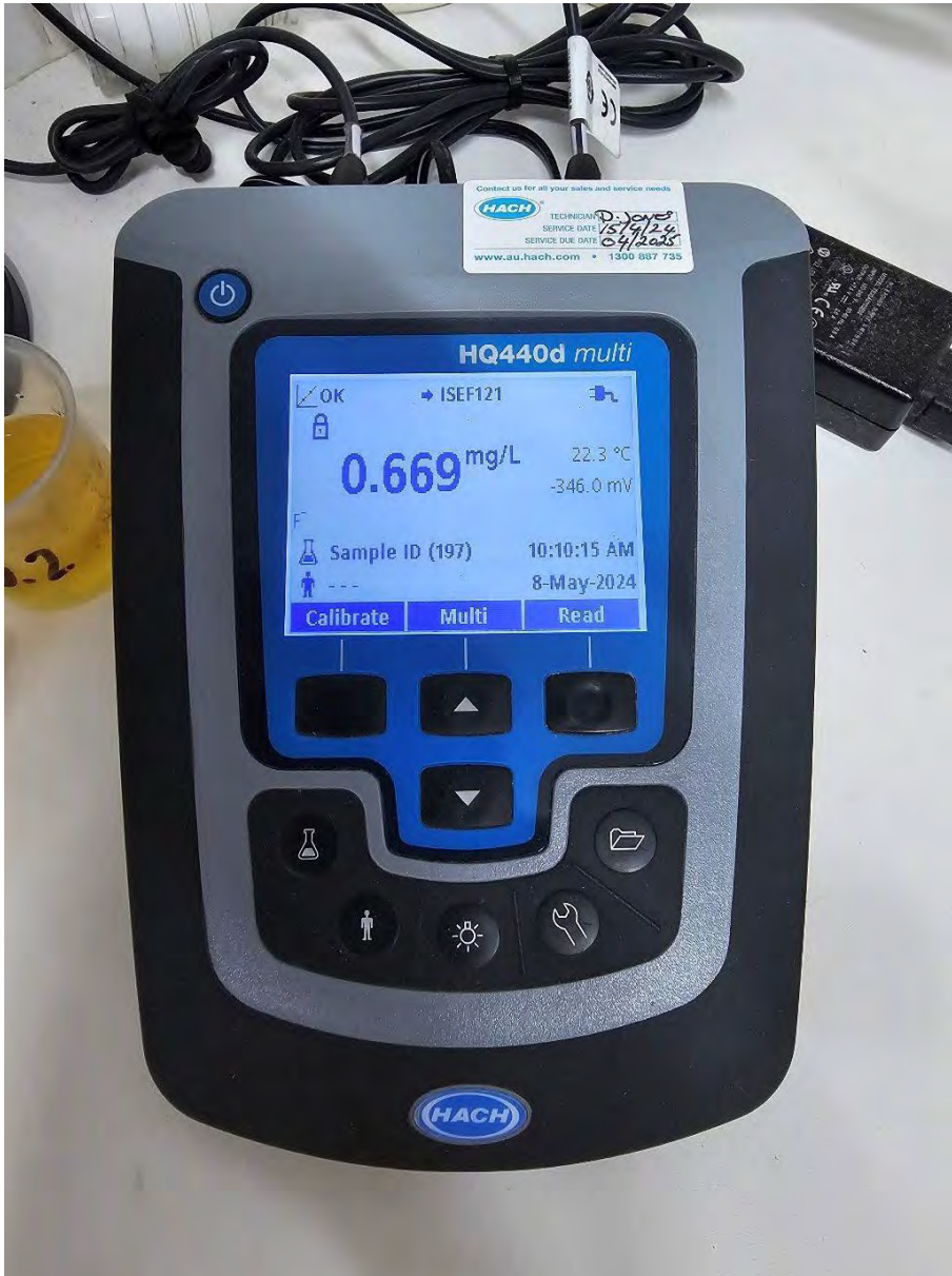
Photo 10: HACH HQ44d – Used by WTP Operator for fluoride testing at Moranbah WTP
