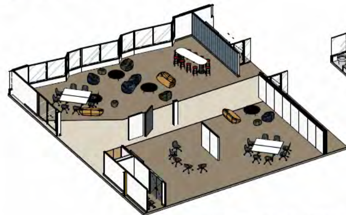
OPERABLE WALL - OPEN CONFIGURATION
